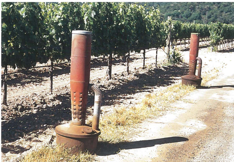
Heaters in Napa County, California. The heat creates air movement, which helps to prevent frosts.
